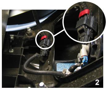
2. Located behind the pumper is a red cap on plug. Slide red cap up then push in to release plug, set plug up out of the way.
