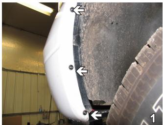
Using a T27 Torx socket remove three torx head bolts from the wheel well just forward the front tire. Do this to both sides and set push pins aside for later reinstallation.
