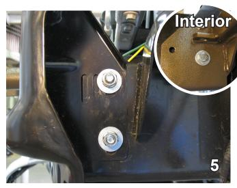
NOTE: Mark the height of bumper bracket on frame.
