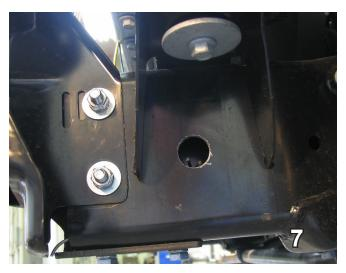
7. Drill 1 1/4" hole with a 1 1/4" hole saw in the center of the frame rail to place nut plates. After making sure bottom hex nut is tight, remove top bolt and use Loctite Red and tighten, then do the same to the bottom hex nut. Do to both sides.
