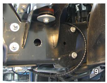
Install the safety cables as directed, around the frame rail suspension support of the vehicle.
