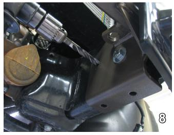
8. Using the baseplate as a template, drill with the 17/32" drill bit the back hole located on the top of the baseplate. Do this to both sides.
