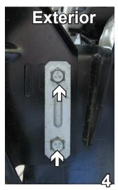
3. Using an 18MM socket, remove three bolts from behind the bumper - two on the bottom, one on the top. Do to both sides and set bolts and bumper aside for later reinstallation.
