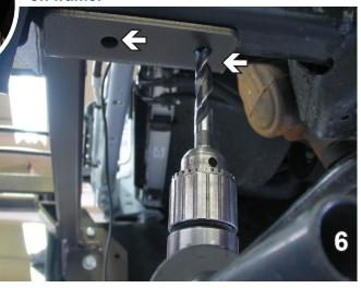
While holding bumper brackets in place align baseplate to the interior hole and insert 1/2-13 x 4" bolts and flat washers on both sides. before tightening, adjust bumper bracket to the previous height, then slide baseplate up to the bottom of the frame and tighten bolt and hex nuts.
