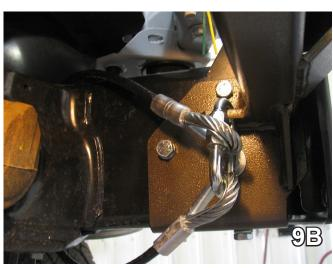
9B. Quick link the safety cables to the convenience link on baseplate. Reinstall fascia. Do this to both sides.
