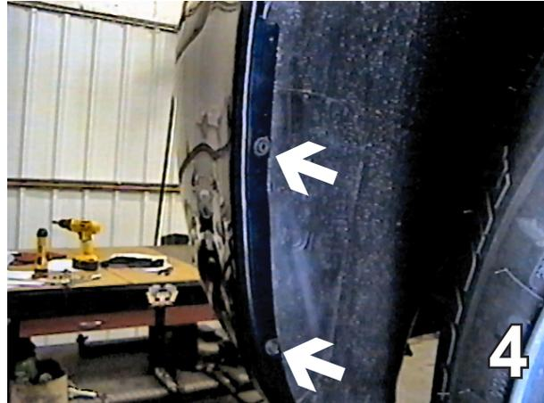
4. Forward of front tires are two screws to remove from wheel well edge with the Phillips screw driver, both sides.
