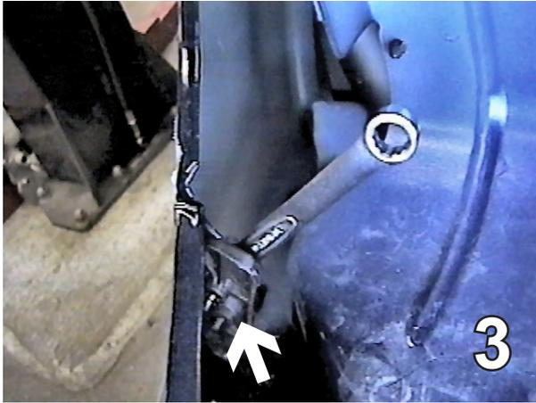
3. Just behind headlight assembly is one metric bolt to remove with the 8MM socket or wrench, both sides.
