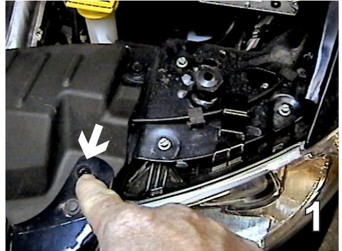
1. Remove one metric bolt just between headlight assemblies on top edge of fascia, with the 10MM socket, both sides.
