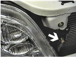
3. Just inside headlight assembly is one metric bolt to remove with the 10MM socket, both sides.
