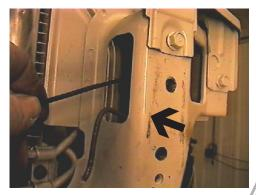
the way through to the back side of radiator cross member, both sides.
