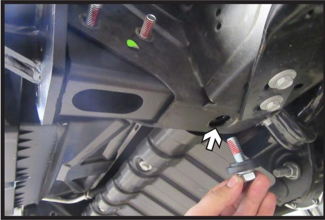
16. Start the bottom 1/2" x 1-3/4" bolt with lock washer, thick washer, and slotted plate. Press baseplate up and in while hand tightening the bolt. Do this on both sides of the vehicle.
