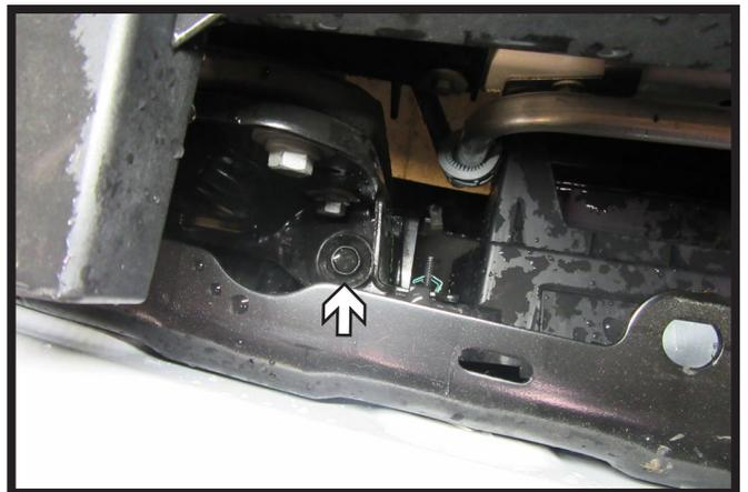
13. On the top side of the bumper, use an 18MM socket with socket extension to remove the one (1) bolt from behind the bumper. Do this on both sides of the vehicle. Remove bumper and set aside to be reinstalled later.
