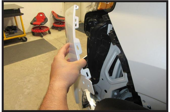
7. Grab fascia in the wheel well and pull outward firmly to remove corner of center fascia piece. Do this on both sides of the vehicle. Lift front center piece upward to release. Remove center fascia piece and set aside to be reinstalled later.
