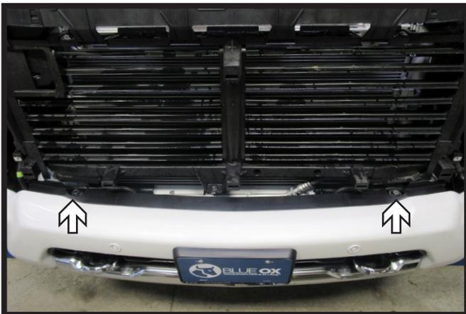
12. Using an 18MM socket, remove the two (2) bolts from the top edge of the bumper. Then remove plastic cover.
