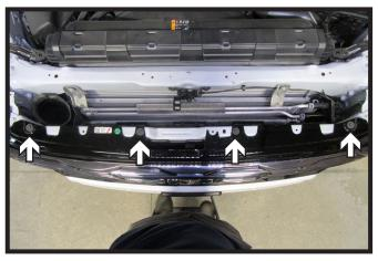
3. Using a 10MM socket, remove the four (4) bolts from the top of the fascia.
