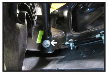
On the underside of the vehicle, use a 15MM socket to remove the one (1) bolt holding the bracket. Do this on both sides of the vehicle.
