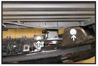
14. Using an 18MM socket, remove the two(2) bolts from the bumper. Do this on both sides of the vehicle. Remove bumper and set aside to be reinstalled later.
