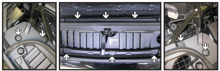
2. Remove the ten (10) push pins from along the top of the fascia. Remove fascia cover and set aside to be reinstalled later.
