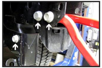
15. Remove the plastic piece from the tow hook. Then using an 18MM socket, remove the three (3) bolts. Do this on both sides of the vehicle. Remove tow hook, it will not be reinstalled later.
