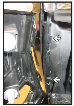
7. Unclip the plastic piece in the center of the headlight by pushing toward the center of the vehicle. Do this on both sides of the vehicle.
