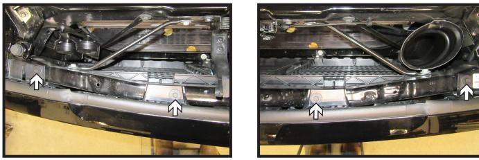
3. Using a 10MM socket, remove the four (4) bolts, two (2) on each side from the top of the fascia.
