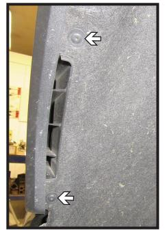
4. Using a T15 Torx, remove the two (2) bolts from the inside of the wheel well. Do this on both sides of the vehicle.
