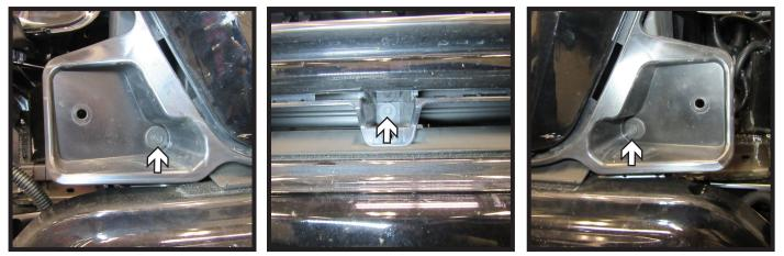
8. Using a 10MM socket, remove the three (3) bolts from the fascia, one (1) in the center and one (1) on each side.
