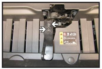
1. Using a T15 Torx, remove the two (2) bolts from the handle on the top edge of the fascia. Remove and set aside to be reinstalled later.
