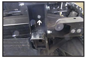
18. Using a 1/2" drill bit, drill the top rear hole on the side of the baseplate (left) and the bottom hole (right), using the baseplate as a template. Do this on both sides of the vehicle.
