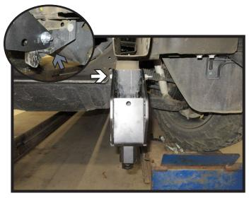
16. Slide baseplate onto tow hook housing so that the back slotted hole of the baseplate lines up with back hole on housing. Insert the one (1) 1/2" x 5" bolt as shown. Leave loose at this time. Do this on both sides of the vehicle.
