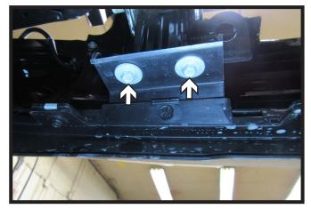
12. Using a 10MM socket, remove the two (2) bolts on the underside of the bumper. Do this on both sides of the vehicle.
