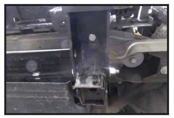
20. Install the 1/2" bolt with hardware into the bottom bolt of the baseplate. Do this on both sides of the vehicle.
