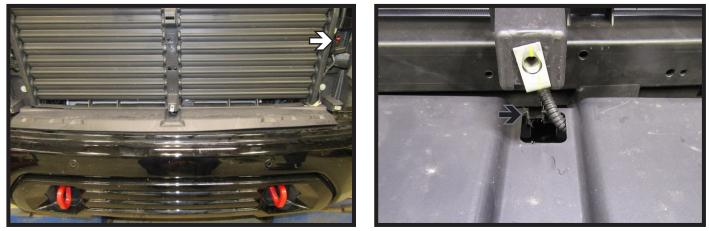
10. Remove seven (7) push pins on the underside of the plastic shroud. Then, either unplug the electrical as indicated (white) or slot the plastic shroud (black) to allow removal. Remove piece and set aside to be reinstalled later.
