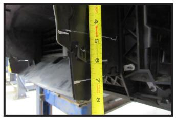
15. Measure down from the bottom of the bumper 4-1/2" and 6-3/4" and mark the shroud. Using a reciprocating saw cut and remove the indicated area.
