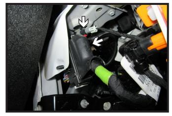
9. Unplug the two (2) electrical connections on the passenger side of the vehicle.
