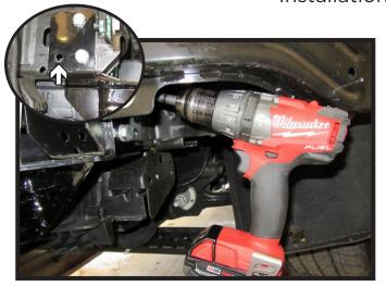
18. Using a 1/2" drill bit, drill the two (2) holes on the driver side and one (1) hole on the passenger side (inset) using the baseplate as a template. Install the remaining three (3) 1/2" bolts with lock washers and whiz nuts into the side plates.
