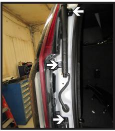
Using a T15 Torx, remove the three (3) bolts attaching the tail light to the vehicle.
