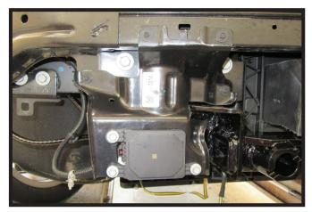
20. **Models with ACC:** Hold ACC bracket up to the vehicle. Mark and trim bracket to allow clearance for the baseplate. Slide the ACC sensor back through hole in bracket and reinstall sensor onto bracket and then bracket onto the vehicle.
