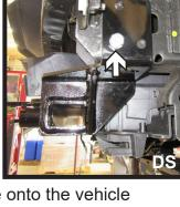
17. Slide the baseplate onto the vehicle and install three (3) 1/2" bolts with lock washers and whiz nuts, two (2) bolts on the passenger side and one (1) on the driver side.
