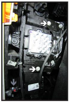
10. Pull back the wheel well liner. Unplug the electrical on the driver side of the vehicle (gray). Using a 10MM socket, remove the two (2) bolts in front of the tire (white). Do this on both sides of the vehicle.
