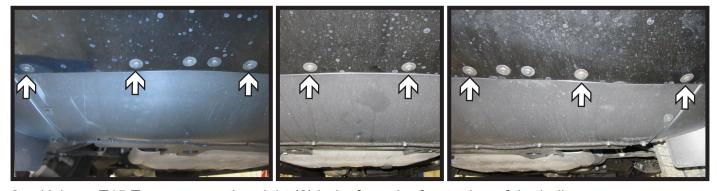
6. Using a T15 Torx, remove the eight (8) bolts from the front edge of the belly pan.
