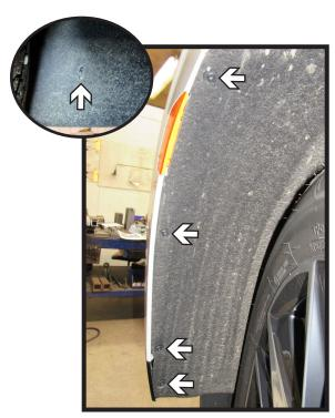
3. Using a T15 Torx, remove the five (5) bolts from the wheel well liner. Do this on both sides of the vehicle.
