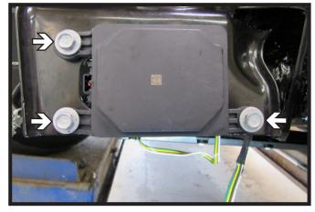
13. **Models with ACC:** Using a 10MM socket, remove the three (3) bolts from the Adaptive Cruise Control (ACC) sensor on the passenger side of the vehicle. Turn sensor and feed it through the hole on the bracket toward the vehicle. Let sensor hang to be reinstalled later.
