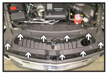
1. Remove the nine (9) push pins from the fascia cover. Remove cover and set aside to be reinstalled later.
