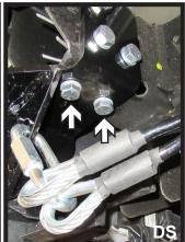
19. Using a 1/2" drill bit, drill the bottom two (2) holes on each side of the vehicle using the baseplate as a template. Then install four (4) 1/2" bolts with lock washers and whiz nuts.
