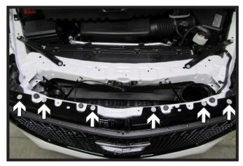
2. Using a 10MM socket, remove the six (6) bolts for the top of the fascia.
