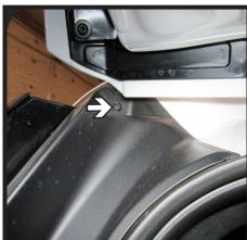
Using a T15 Torx, remove the one (1) bolt at the top of upper plastic cover.
