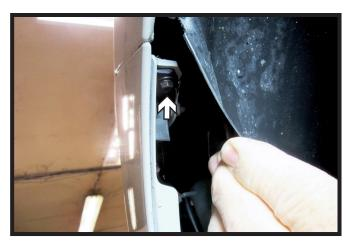
Pull back the wheel well liner. Using a 7MM socket, remove the one (1) bolt from the fascia joint. Do this on both sides of the vehicle.
