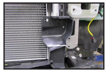
Measure down approximately 3-1/2" from the top of the shielding and cut thru the plastic shielding. Discard the upper portion of the shielding. Do this on both sides of the vehicle.
