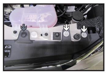
1. Using a 10MM socket, remove the four (4) bolts (white) from the top of the fascia. Then remove the two (2) push pins (gray).
