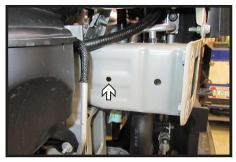
Using a 3/8" drill bit, drill out the back hole in the frame on the passenger side of the vehicle.
