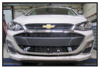
14. Hold the fascia as close to its original position, mark and trim the fascia around the convenience links, attachment tabs and optional breakaway switch. Reinstall the fascia and reconnect all electrical.
