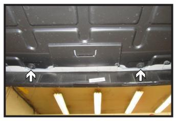
4. Using a 7MM socket, remove the eight (8) bolts from the underside of the fascia. There are three (3) on each side and two (2) in the middle. Remove fascia, disconnecting any electrical connections, and set aside to be reinstalled later.
