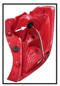
Drill a hole according to the tail light wiring kit instructions.
