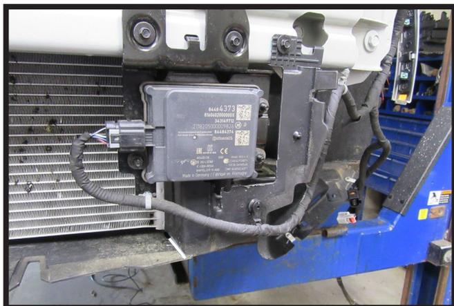
8. Unsnap the ACC wire loom from the shutter housing and bumper on the driver side of the vehicle.
