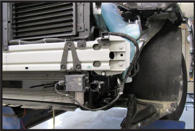
18. Reinstall the ACC and the windshield washer fluid reservoir on the driver side of the vehicle.
