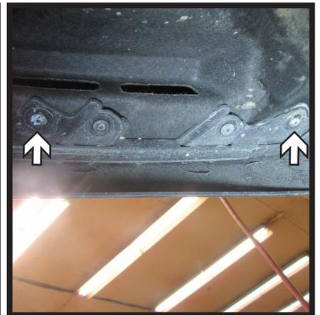
5. Using a T15 Torx, remove the eight (8) bolts from the underside of the fascia. There are two (2) on each side and four (4) in the middle.
