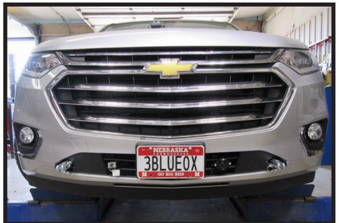
21. Hold the fascia as close to its original position, mark and trim the fascia around the convenience links and attachment tabs. Use a 2" hole saw to create the initial holes for the attachment tabs. Then trim as needed for the convenience links. Reinstall the fascia, fascia cover, and reconnect all electrical connections.
