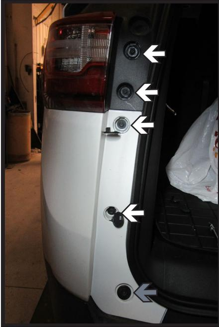
1. Unpop the covers for the five (5) bolts on the back panel of the vehicle. Then using a 7MM socket, remove the four (4) top bolts (white) and a T20 Torx socket to remove the one (1) bottom bolt (gray). Do this on both sides of the vehicle.
