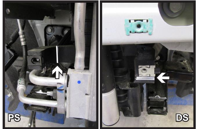
11. Using a reciprocating saw, trim the brackets on the driver and passenger sides of the vehicle as indicated to allow clearance for the baseplate.
