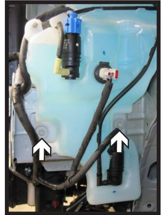
7. On the driver side of the vehicle, using a 10MM socket, remove the one (1) nut from the top of the windshield washer fluid reservoir. Disconnect all lines. Then using a 10MM socket, remove the two (2) bolts at the bottom of the reservoir.
