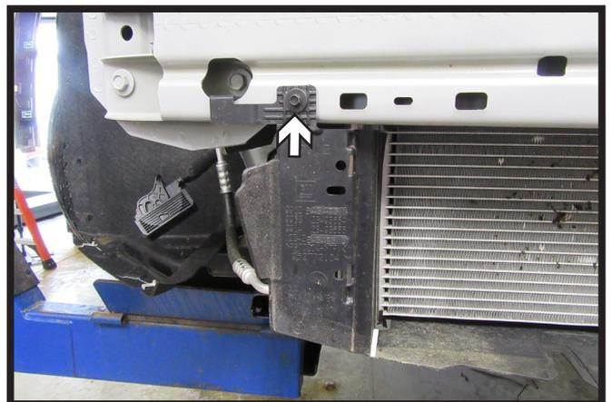
9. Using a 7MM socket, remove the two (2) bolts, one (1) on each side from the shutter housing. Using a utility knife remove the side pieces of the shutter housing as indicated.
