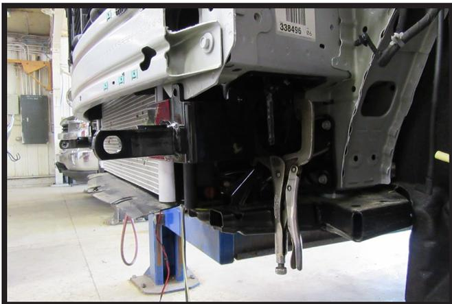
12. Slide baseplate into place. Use large vise grips to hold in place. Do this on both sides of the vehicle.
