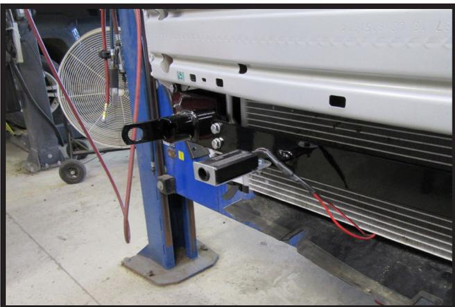
20. **Optional Breakaway:** Attach the breakaway switch to the bracket on the passenger side of the vehicle using the 1/4" hardware.
