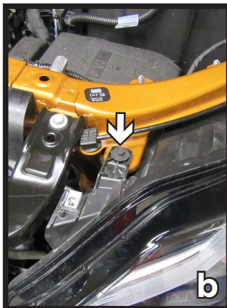
7. Using a 7MM socket, remove the four (4) bolts attaching the driver side head light. Remove and set aside to be reinstalled later.
