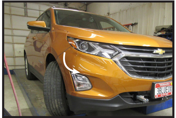
6. Pull the corners of the fascia away from the vehicle. Disconnect all electrical connections and pull the fascia from the vehicle. Set aside to be reinstalled later.
