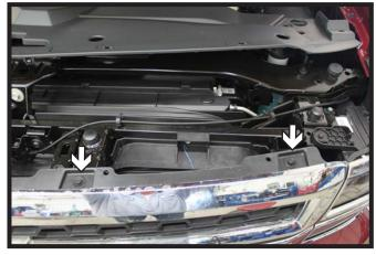
Using a 10MM socket, remove the four (4) screws from the top edge of the fascia. There are two (2) on each side.
