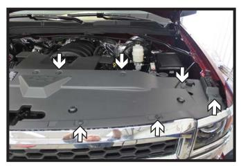
1. Remove the twelve (12) push pins from the fascia cover. There are six (6) on each side. Set the cover aside.
