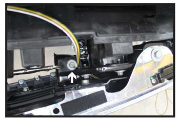
12. Reinstall the bumper onto the vehicle. Install the top outer bolts, then push in on the bottom of the bumper to line up the inner bottom bolts. Clamp the bumper when the hole is lined up and reinstall the lower bolts. Continue to reinstall the bumper bar bolts and reconnecting the electrical connections on the underside of the bumper.
