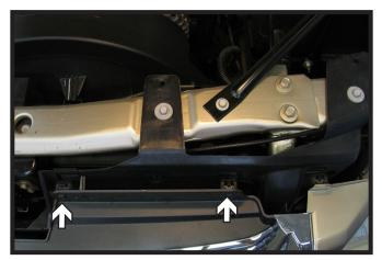
1. Release the four (4) snaps from the top edge of the grille. There are two (2) on each side.
