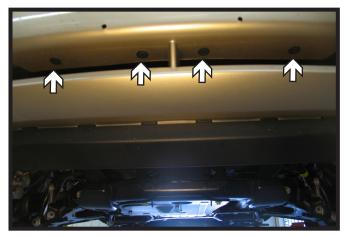
On the underside of the lower fascia opening, remove the four (4) push pins. Remove the fascia from the vehicle.
