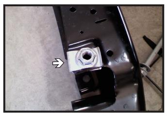
Remove the factory nut bracket from the bumper. Do this on both sides of the bumper.
