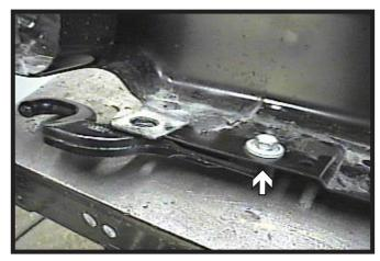
If equipped, using a 15MM socket, remove the tow hooks. The tow hooks will not be reinstalled.
