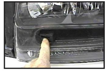
Trailblazer Only: The grille is also attached towards the middle of the headlight assembly. Pull forward to release the clip. Do this on both sides of the vehicle and set the grille aside.
