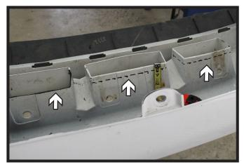
16. Trailblazer Only: On the backside of the fascia, trim the middle three (3) openings approximately as shown for baseplate clearance.
