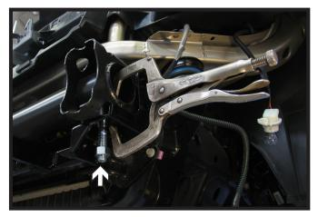
11. Position the baseplate onto the vehicle. Install the 5/8"-11 x 8" bolt thru the frame and baseplate to position it on the frame and clamp in place.
