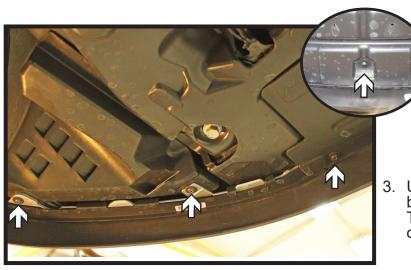
3. Using a T20 Torx, remove the seven (7) bolts from the underside of the fascia. There are three (3) on each side and one (1) in the middle (inset)
