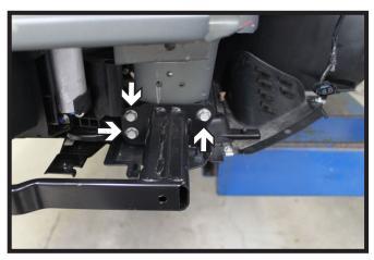
8. Using a 13MM socket, remove the three (3) bolts from the lower fascia support. Do this on both sides of the vehicle. Set the support aside.
