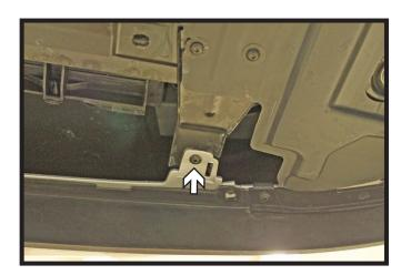
Using a Phillips screwdriver, remove the two (2) screws that are now visible after the removal of the belly pan. There is one (1) on each side.
