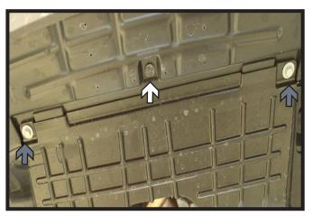
4. On the belly pan, remove the one (1) push pin (white) and with a 13MM socket, remove the two (2) bolts (gray).
