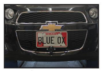
18. Hold the fascia as close to its original position, mark and trim the fascia around the convenience links and attachment tabs.
