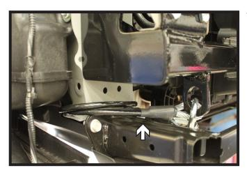
15. Attach the permanent baseplate safety cables to the provided convenience link on the baseplate. The photo above shows the recommended installation of the cables to frame of vehicle. Additional options may interfere with suggested mounting; in this case, secure the cables to a solid piece of the frame as described in the General Instructions. Be sure the safety cables do not rub against any hoses or moving parts. Do this on **BOTH** sides of the vehicle.
