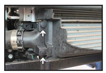
10. **RS-Models:** Remove the two (2) push pins from the plastic shroud. Do this on both sides of the vehicle. Set the shroud aside it will not be reinstalled.
