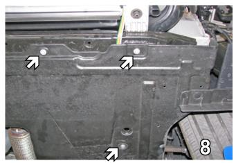
Using an 8MM socket, remove two (2) metric bolts across the front of the belly pan and another across from the tire. Do this on both sides. Set bolts aside to be reinstalled later.
