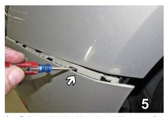
5. Pull out and to the side on the outside corner of the fascia next to the wheel to release the first tab. Using a small flat screwdriver push in on each of the four (4) tabs as you pull the fascia. Do this on both sides. Remove the fascia and set aside carefully to be reinstalled later.
