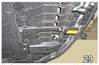
29. Optional: Attach the breakaway and the bracket to the underside of the vehicle with 1/4"-20 x 3/4" bolt and 1/4"-20 hex nut (white arrow). Cut opening in lower air dam to allow front of breakaway to come through (gray arrow).
