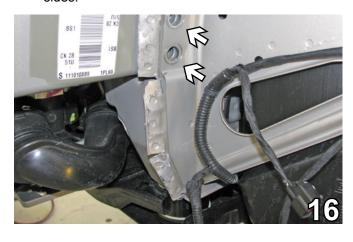
16. Using an 18MM socket and a wrench on the other side, remove the two (2) metric bolts next to the flattened area. Do this on both sides.
