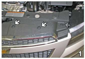
Remove the two (2) push pins (white arrows) from the black plastic cover just above the radiator. Using a 10MM socket, remove the metric bolt at the edge of the fascia (gray arrow). Do this on both sides. Set pins and bolts aside to be reinstalled later.
