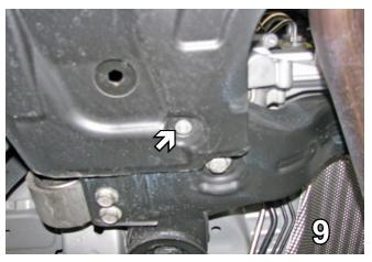
Using an 8MM socket, remove one (1) more metric bolt toward the back of the belly pan. Do this on both sides. Set bolts aside to be reinstalled later.
