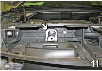
11. Using a 10MM socket, remove the metric bolt from the top of the air intake tube. Set the bolt aside to be reinstalled later.
