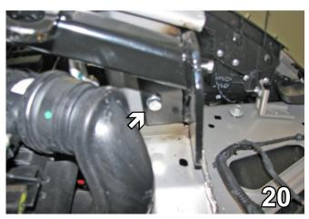
20. Using the baseplate as a template, drill a hole on the bottom side with the 13/32" drill bit. Insert 3/8"-16 x 1-1/2" hex bolt with Loctite Red and 3/8" lock washer. Attach to 3/8" nut plate inserted through the 1-1/2" lower opening on bumper. Do this to both sides.
