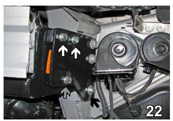
22. Bolt the upper two (2) holes (white arrows) with 3/8"-16 x 2" hex bolts, 3/8" lock washers and fasten to 3/8" nut plates inserted through the drilled hole in the bumper. In the lower outside hole (gray arrow) bolt the support plate to the baseplate with 3/8"-16 x 1-1/2" hex bolt fastened with 3/8" lock washer and 3/8"-16 hex nut. Be sure to use Loctite Red on all bolts. Do this on both sides.
