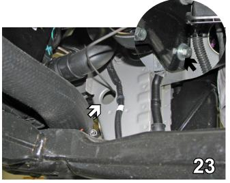
23. Insert 3/8"-16 x 1-1/2" hex bolt with 3/8" lock washer into the lower inside hole on the baseplate (black arrow step 22). Fasten to a 3/8" nut plate inserted through an existing hole underneath in the frame (white arrow). Do this on both sides. Be sure to use Loctite Red on the bolts.
