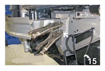
15. Using vice grips, bend the frame webbing over and flatten with a hammer. Do this on both sides.
