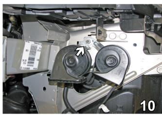
Using the 13MM socket, remove the metric bolt from the horn bracket on the driver side, unplug and set the bolt and horn aside to be reinstalled later.
