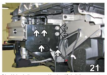
21. Using bolts removed in step 16, bolt the support plates to the existing holes on the outside of the frame (gray arrows). Use 18MM socket and a wrench on the other side to tighten bolts in order to sandwich the baseplate between the frame and the support plates. Using the support plate as a template, drill the other four (4) holes with a 13/32" drill bit (white arrows). Do this on both sides.
