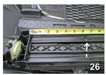
26. On the backside of the fascia, locate the top louver of the air shutter system, measure and mark over 6-1/2" from the left end of the air shutter system. Using the diagonal cutters, make a vertical cut across the louver and remove the 6-1/2" end portion. Do this to both sides of the vehicle. Driver side is shown.
