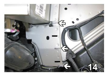
14. Cut frame webbing at the top, at the bend and at the bottom with a reciprocating saw. Be careful not to cut the main part of the frame. Do this on both sides.
