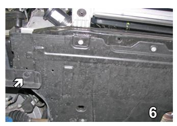
6. Remove one (1) push pin from the bottom of the belly pan. Do this on both sides. Set push pins aside to be reinstalled later.
