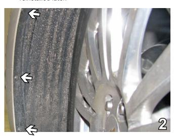
2. Just forward of front tire, on the edge of the wheel well, are three (3) bolts to remove with the T20 Torx, both sides. Set bolts aside to be reinstalled later.
