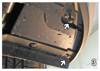
Remove the two (2) bolts from underneath the fascia, just forward of front tires with the T20 Torx, both sides. Set the bolts aside to be reinstalled later.
