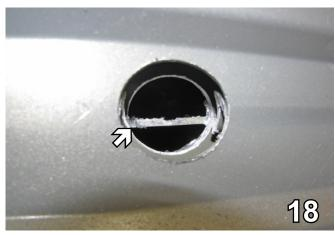
18. Inside the 1-1/2" drilled hole is a cross piece, which may need to be bent vertically with a pry bar in order to insert 3/8" nut plate. Do this on both sides.
