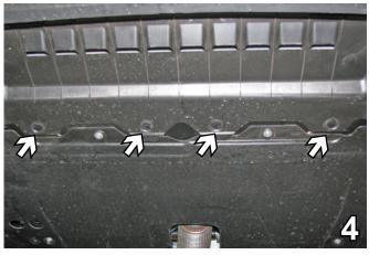
1. Remove the four (4) push pins from underneath the fascia. Set pins aside to be reinstalled later.
