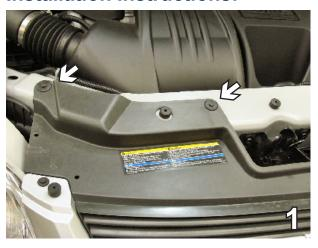
Remove the two push pins from the black plastic cover just above the radiator, both sides.
