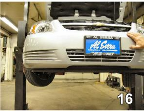
16. Hold fascia as close to its original position as possible, mark and cut the top style of the lower grill opening, on both sides of the attachment tab receivers to allow tabs to come through. Reinstall fascia. Be sure all electrical components are plugged in properly.
