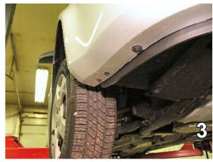
3. Remove the two metric bolts from lower edge of fascia, just forward of front tires with the 7MM socket, both sides.
