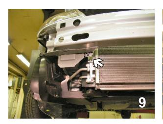
Mark a line from inner edge of bumper brace, along the bottom edge of metal bumper and down, flush with the inside edge of frame rail, both sides (view of passenger's side). Remove this area with the reciprocating saw, both sides.
