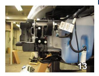
Reinstall horn bracket on the driver's side, using the existing equipment with the 10MM socket. Be sure that all electrical connections are plugged in properly.
