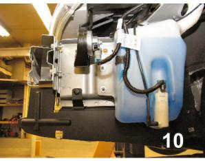
Using the 10MM socket, remove the metric bolt from the horn bracket on the driver's side, unplug and set aside.
