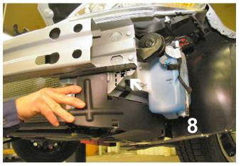
8. Mark a line from outer edge of bumper brace, along the bottom edge of metal bumper and down, flush with the outside edge of frame rail, both sides (view of driver's side). Remove this area with the reciprocating saw, both sides.
