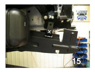
15. Mark a line on the bottom edge of the tab that connects to the intake tube front bolt location and mark a line on the air dam just below metal bumper, both sides. Cut and remove these two areas with the utility knife, both sides.
