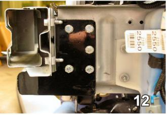
12. Using the baseplate as a template, drill four holes on the driver's side and the four holes on the passenger's side with the 13/32" drill bit. Insert the nut plates into the end of frame rail, just behind metal bumper bracket to align with drilled holes, insert 3/8-16 x 1 1/2" hex bolts and lock washers into baseplate/drilled holes with the 9/16" socket, both sides.
