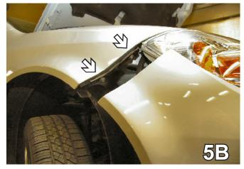
5. Remove the lower metric bolt just forward of the front tire (left photo), on fascia's upper corner, using the 10MM socket, both sides. Loosen the top and bottom remaining metric bolts to release fascia's corner, with the 10MM socket, both sides.
