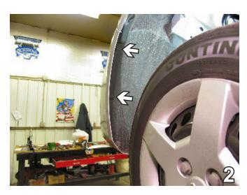
Just forward of front tire, on edge of wheel well, are three metric bolts to remove with the 7MM socket, both sides.
