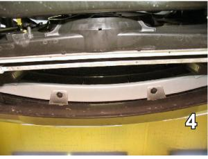
4. Remove the two push pins from the fascia tabs, just below metal bumper, behind fascia.
