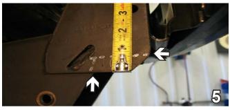
5. Using a reciprocating saw, cut along the ridge 3/4" up and straight across to remove the piece. Do this to both sides of the vehicle.
