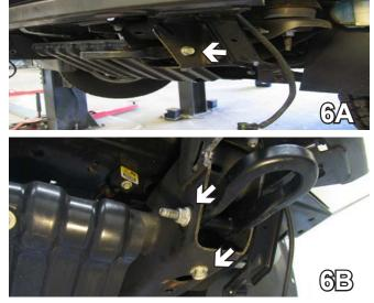
Using a 18MM socket, remove one bolt from the side and one bolt from the bottom of the tow hook. Do this to both sides of the vehicle. Factory tow hooks and bolts will not be reinstalled.
