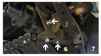
7. Slide baseplate in where the tow hooks were removed. Insert a 1/2-13 x1 1/4" hex bolt with loctite and 1/2" lock washer into the two holes on the side and the two holes on the bottom of the baseplate and tighten bottom two down first. Do this to both sides of the
