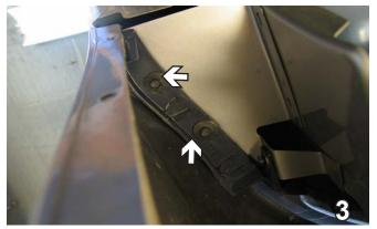
Using a 10MM socket, remove two bolts located just behind the wheel well plastic that we removed the bolts and push pins from. Do this to both sides of the vehicle. Set bolts aside to be reinstalled later.
