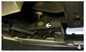
Using a 10MM socket, remove one bolt located underneath the fascia just left of the frame. Do this to both sides of the vehicle. Pull the fascia forward to remove. Set fascia and bolts aside to be reinstalled later.
