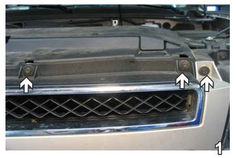
1. Remove three bolts with a 10MM socket. Do this to both sides of the vehicle. Set bolts aside to be reinstalled later.
