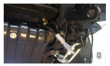
8. The photo above shows the recommended installation of the cables to frame of vehicle. If vehicle has additional options (not shown above) which interfere with mounting permanent baseplate safety cables, secure the cables to a solid piece of the vehicle frame as described in instructions included with the permanent baseplate safety cables.
