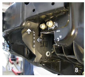
8. Using a flat screwdriver, remove push pin (see white arrow) and then using a utility knife, cut along dashed line shown in the photo above (see grey arrow). The plastic piece will not be reinstalled and can be discarded. Do this to both sides of the vehicle.
