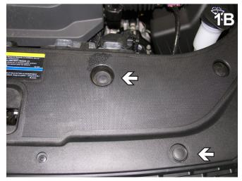
1. Using a flat screwdriver, remove three push pins from the flat plastic piece on top. Do this to both sides of the vehicle. Set push pins aside to be reinstalled later.
