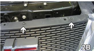
2. Once top piece is set aside, you will need to remove three (3) screws with a Phillips screwdriver and one (1) push pin with a flat screwdriver. Do this to both sides of the vehicle. Set screws and push pin aside to be reinstalled later.
