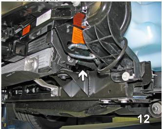
12. Attach the permanent baseplate safety cables to the provided convenience link on the baseplate. Secure the cables to a solid piece of the frame as described in the instructions included with the permanent baseplate safety cables. Be sure the safety cables do not rub against any hoses or moving parts. Do this to both sides of the vehicle.
