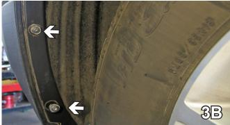
Using a Phillips screwdriver, remove five
