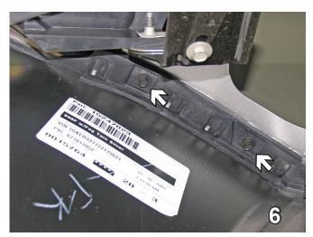
6. You will then need to pull plastic back underneath and remove two (2) metric bolts with a 7MM socket. Do this to both sides of the vehicle. Set bolts aside to be reinstalled later. The fascia is then ready to be removed from the vehicle and set aside carefully to be reinstalled later.
