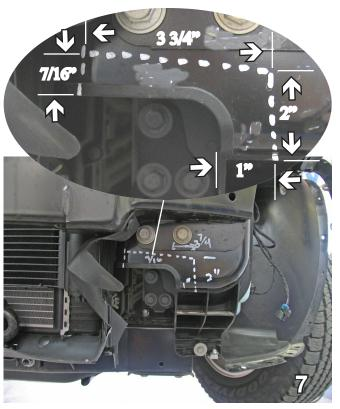
7. Mark and cut out frame according to the photo above, using a reciprocating saw. Do this to both sides of the vehicle.
