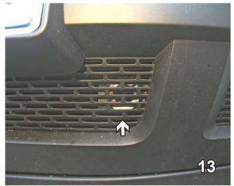
13. Align the fascia to its original position and using a hack saw blade, remove area around attachment tab receiver to allow for it to come through fascia. Do this to both sides of the vehicle.
