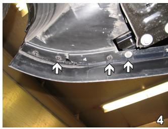
4. Located just forward the front tire underneath, you will need to remove two (2) screws with a Phillips screwdriver and one (1) bolt with a 10MM socket. Do this to both sides of the vehicle. Set screws and bolts aside to be reinstalled later.
