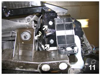
11. Using the baseplate as a template, drill the two (2) bottom holes into the frame with a 17/32" drill bit. Insert the 1/2" nut plates into the frame and align with drilled holes. Insert a 1/2"-13x1-1/2" hex bolt and 1/2" lock washer into each hole and tighten down with Loctite Red. You will then need to finish tightening down the front two (2) bolts. Do this to both sides of the baseplate.
