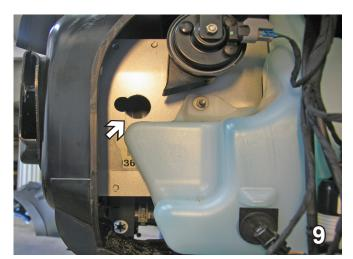
9. Drill a 1-1/4" hole into the frame, so the nut plates can go through. Do this to both sides of the vehicle.
