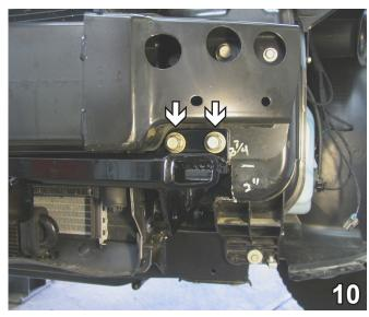
10. Using a 15MM socket, remove two (2) bolts from the front of the bumper. Do this to both sides of the bumper. Slide baseplate straight back, so that the holes on the baseplate line up with the existing holes of the bumper. Reinsert the existing bolts and tighten down, so the bolts are snug. Do this to both sides of the baseplate.
