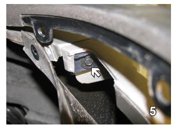
Once screws are removed from wheel well, pull plastic back on top and remove one (1) metric bolt with a 7MM socket.
