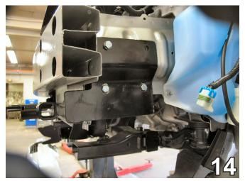
14. Using the baseplate as a template, drill the remaining three holes into the frame rail on the driver's side with the 13/32" drill bit. Insert two 3/8-16 x 1 1/2" hex bolts, 3/8-16 hex nuts and 3/8 lock washers into the bottom two holes. Guide a 3/8" nut plate up through the opening in the bottom of the frame rail and align it with the upper front bolt hole. Install the 3/8-16 x 1 1/2" hex bolt and the 3/8" lock washer to the 3/8-16 nut plate.
