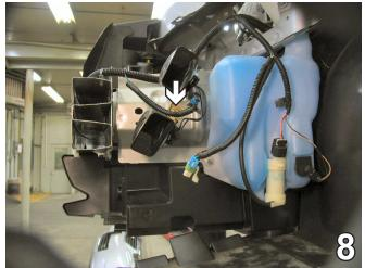
8. Using the 10MM socket, remove one metric bolt from the driver's side horn bracket. Disconnect the horn. Set bolt, bracket, and horn aside to reinstall later.
