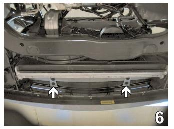
6. Remove two pushpins from the fascia tabs. Do this to both sides of the vehicle. Set pushpins aside to reinstall later.
