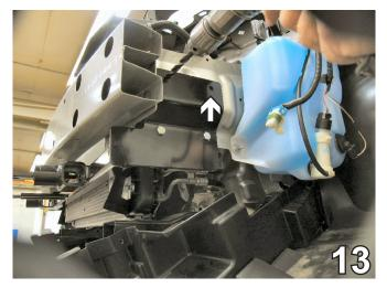
13. Align the baseplate on the driver's side so the upper back hole aligns with the existing horn bracket hole and clamp in place with vise grips.
