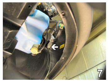
7. Using the 10MM socket, remove one metric bolt from the corner of the fascia, just forward of the front tires, inside the headlight assembly. Do this to both sides of the vehicle. Set bolts aside to reinstall later.
