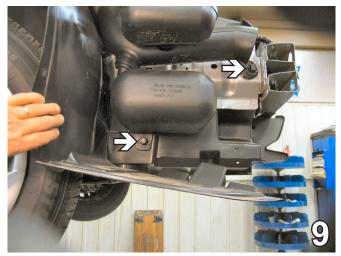
9. Remove two pushpins from the passenger's side air baffle. Set bolts and air baffle to reinstall later.
