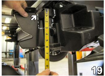
On the driver's side, just behind the tab of air dam, cut down three inches. Then, cut horizontally toward rear of air dam approximately two inches. Cut upwards to the top, following the contour of the air dam.
