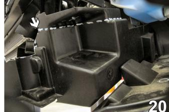
20. On the driver's side, approximately one inch from the top of the air dam, cut horizontally from the front of the air dam to the back.
