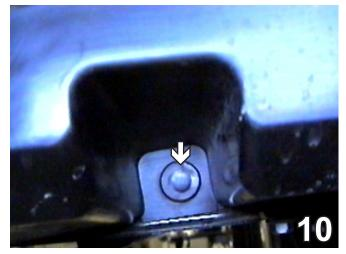
10. Remove one push pin from the lower plastic on the bottom rib of the frame rail. Do this to both sides of the vehicle. Set pushpins aside to reinstall later.
