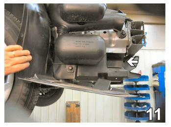
11. Remove one pushpin from the passenger's side of the air dam. Pull air dam down to clear area for baseplate installation. Set bolt aside to reinstall later.
