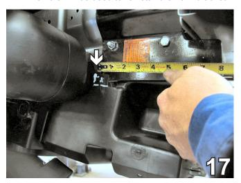
17. On the passenger's side upper rear of the air dam, use the utility knife to make a one inch horizontal cut level with the opening next to the air dam then trim vertically to remove this portion of the air dam.
