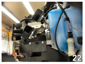
22. Using the 10MM socket, secure the horn bracket using a 6 x 1 x 30MM hex bolt with 1/4" lock washer and 1/4" flat washer.
