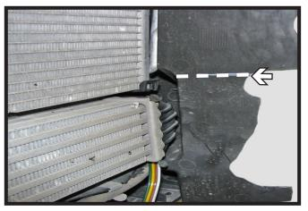
18. Trim the lower portion of the plastic shrouding off as shown for baseplate clearance. Do this on both sides of the vehicle
