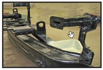
15. Set the bumper upside down on a table. Holding the baseplate upside down, insert the passenger side first (white arrow). Then slide the driver side into place on the bumper extension. The baseplate should be positioned as far forward as possible and then securely clamp in place.
