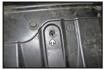
23. **Optional:** Attach the breakaway to the bracket with 1/4"-20 x 3/4" bolt and 1/4"-20 nut (left). Insert the breakaway switch into the grille opening in line with the center bolt hole on the driver side of the fascia cover. Reinstall the grille and the cover. Attach the breakaway bracket with an existing bolt inserted from the top of fascia cover that was removed in step 1 (right).
