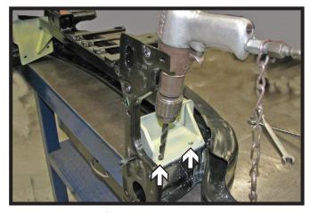
16. Using a 13/32" drill bit, drill the bottom two (2) holes in the baseplate thru the bumper. Install 3/8"-16 x 1-1/4" bolts with 3/8" lock washers into the holes and 3/8"-16 nut plates.
