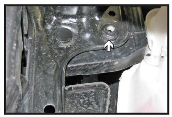
13. Using a 16MM socket, remove the bolt from the backside of the middle bumper bracket. Do this on both sides of the vehicle.
