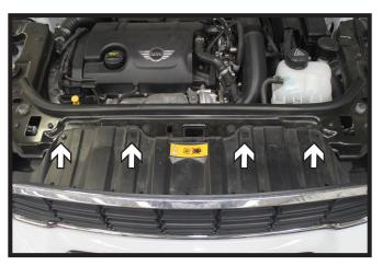
Using a 10MM socket, remove the four (4) screws from the fascia cover and set aside.
