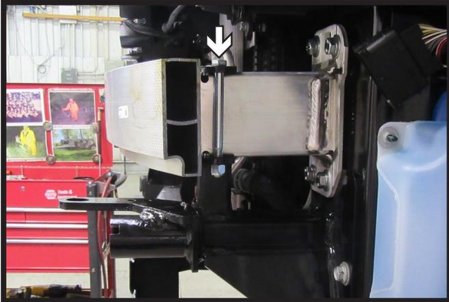
15. Place bracket on top of the bumper and secure to baseplate using two (2) 3/8" x 4-1/2" bolts with nylon lock nuts. Do this on both sides of the vehicle.
