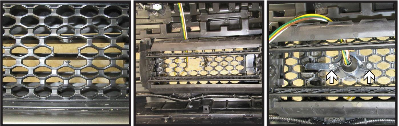
18. **Shutter Models:** Trim the fascia as shown on one side of the vehicle to allow room for the electrical (left). On the back side of the fascia remove the middle shutter to allow room to attach electrical bracket (center). Set aside shutter to be trimmed and reinstalled later. Cut a hole in the top of the shutter housing to run electrical through and install electrical bracket using two (2) 1/4" bolts with hardware (right).
