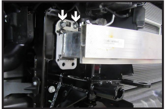
12. Reinstall bumper with spacer plate between the frame and the top of the bumper. Start the two (2) 10MM bolts with flat washers and lock washers. Do this on both sides of the vehicle.
