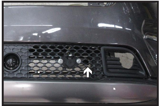
20. **Optional:** Trim fascia to allow room for breakaway switch. Attach breakaway switch to the electrical mounting bracket using one (1) 1/4" bolt and nut (gray).
