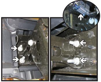
Using an 18MM socket, remove the four
