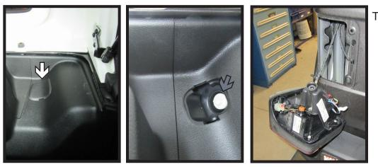
Tail Light Removal: Remove the cover (white) in the back inside of the vehicle. Using a 10MM socket remove the nut (gray). The tail light can now be pulled out of the housing. Do this on both sides of the vehicle.
