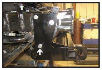
Install the 1/2" bolt with lock washer and whiz nut into the bottom hole on the outside of the frame. If the hole does not completely line up ream out hole with drill bit. Do this on both sides of the vehicle.
