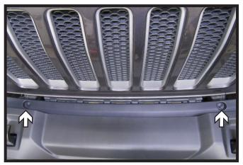
Remove the two (2) push pins, directly behind the tow hooks, from the plastic piece between the bumper and the grille. Remove and set aside to be reinstalled later.
