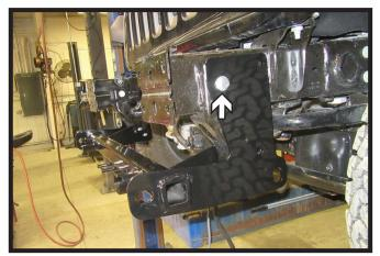
Slide the baseplate onto the vehicle. Start the front 10MM bolt with flat washer and lock washer. Snug bolt up tight so remaining holes line up but do not use Loctite<sup>®</sup> Red at this time. Do this on both sides of the vehicle.
