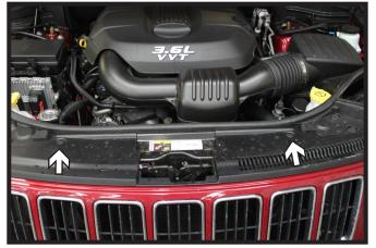
On the topside of the fascia, remove the two (2) push pins.
