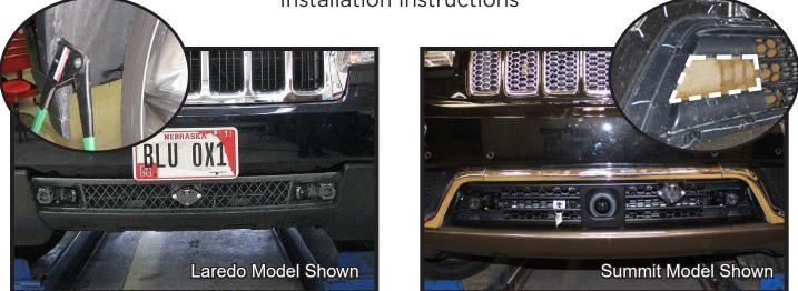
16. Hold the fascia as close to its original position as possible, mark and trim the fascia around the convenience links and attachment tabs. Reinstall the fascia. Using the plastic pop rivet gun, replace the two (2) rivets in the wheel well. Do this on both sides of the vehicle.
