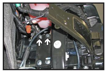
Using a 3/8" drill bit, drill the top two (2) holes of the support plate thru the frame. Install 3/8"-16 x 1-1/4" bolts with 3/8" lock washers and 3/8"-16 lock nuts. Do this on both sides of the vehicle. Fully tighten all hardware.
