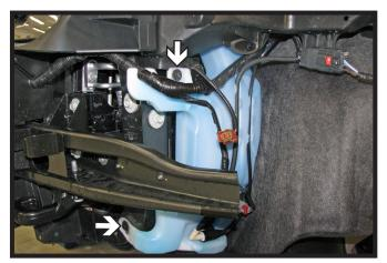
Using a 8MM socket, remove the two (2) bolts from the washer fluid reservoir. Disconnect/plug all lines and set reservoir aside.
