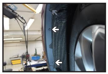
2. Using a utility knife, remove the two (2) plastic rivets from outer edge of the wheel well (white). Then using a 10MM socket, remove the upper screw (gray). Do this on both sides of the vehicle.
