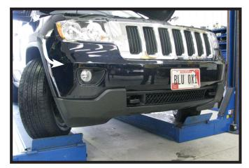
Pull the top corners of the fascia out releasing the clips behind. Continue working inward towards the grille releasing the clips under the headlights and grille. Set the fascia aside to be reinstalled later.
