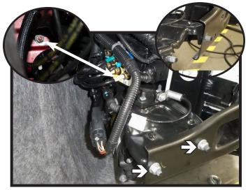
4. On models equipped with a compressor, using a 10MM or 13MM socket, remove the two (2) nuts from the bumper and one (1) nut from the frame behind the compressor (left inset). Move the compressor away from the frame. Put the inner stud into the outer bumper hole and thread on a nut to secure in position (right inset). This will allow room for baseplate installation.
