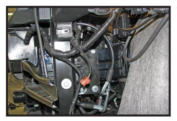
11. Attach the permanent baseplate safety cables to the provided convenience link on the baseplate. The photo shows the recommended installation of the cables to frame of vehicle. Additional options may interfere with suggested mounting; in this case, secure the cables to a solid piece of the frame as described in the General Information sheet. Be sure the safety cables do not rub against any hoses or moving parts. Do this on **BOTH** sides of the vehicle.
