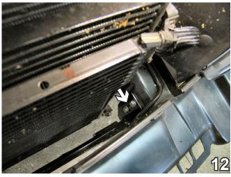
12. Install the 3/8-16 x 1 1/4" hex bolts with 3/8" lock washers into the drilled holes. Insert 3/8-16 nut plates into the frame rail opening and align with the bolts. Tighten all bolts. Do this to both sides of the vehicle.
