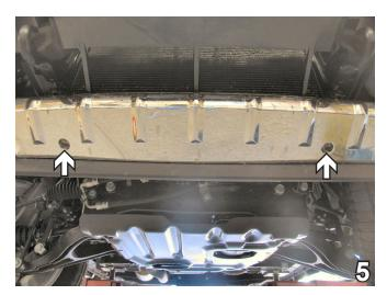
Using a 10MM socket, remove two metric bolts on the bottom side of the fascia. Set bolts aside to be reinstalled later.
