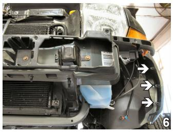
6. Release the three clips from inside of the wheel well, just forward of the front tire, on the fender guard. Disconnect fog lights (if applicable). Pull forward on the fascia and set it aside carefully to be reinstalled later.
