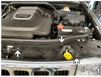
Remove six pushpins from the top of the fascia. Set pushpins aside to be reinstalled later. The driver's side is shown.
