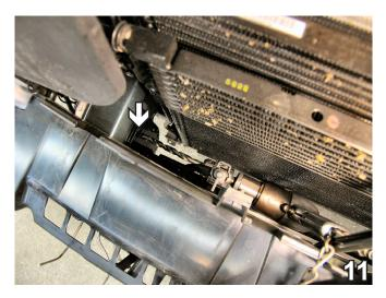
11. Using the baseplate as a template, drill two holes into the frame rail, between the radiator and the metal bumper, with the 13/32" drill bit. Do this to both sides of the vehicle.
