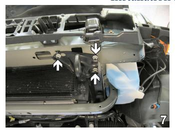
Using a 15MM socket, remove three metric nuts from the tow hook. Do this to both sides of the vehicle. The tow hooks will **NOT** be reinstalled, make sure that these are returned to the customer.
