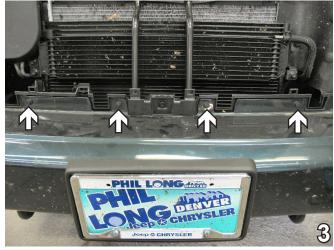
Remove four pushpins from the top of front fascia. Set pushpins aside to be reinstalled later.
