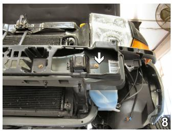
8. Using a 10MM socket, remove the metric nuts securing the frame rail cup to the frame. Do this to both sides of the vehicle. Set nuts and cup aside to be reinstalled later. Remove the factory installed nut plate for the tow hook, found in the opening behind the frame cup. Set the nuts and nut plates aside to be reinstalled later. Do this to both sides of the vehicle.
