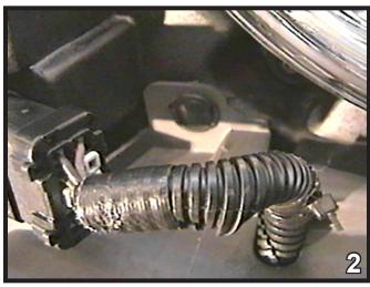
2. Remove the six push pins from the top side of the fascia. Disconnect the electrical plug on the driver's side as seen in the photo above.
