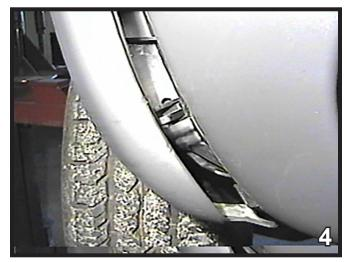
Release three clips from the fascia's side by opening the access panel on the wheel well, just forward of the front tires. Do this to both sides of the vehicle.
