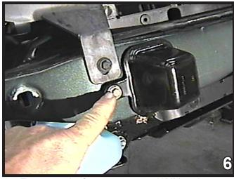
6. To remove the frame cup, use a 10MM socket to remove the metric bolt. Set cup and bolt aside to be reinstalled later. Do this to both sides of the vehicle. Some models may have tow hooks that will be removed at this time.
