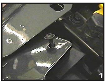
Using the T-20 Torx, remove the two Torx bolts from the top of the headlight assembly and two on the top center of grille. Do this to both sides of the vehicle. Set the torx bolts aside to be reinstalled later. Pull top of grille forward and lift up to remove.
