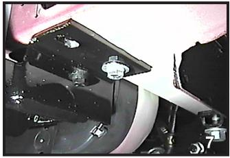
BE SURE TO USE LOCTITE® RED ON ALL BOLTS BEFORE TIGHTENING. TIGHTEN ALL BOLTS ACCORDING TO THE TORQUE CHART ON THE FRONT PAGE OF THESE INSTRUCTIONS OR ON PAGE 3 OF THE BASEPLATE TOWING GENERAL INSTRUCTIONS.
