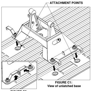
FIGURE C2: View of closed latch handle
