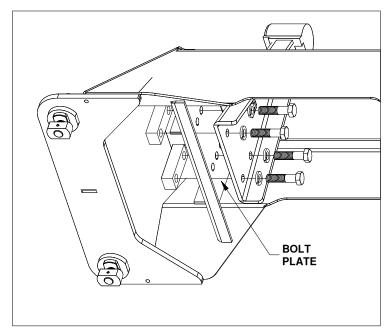
FIGURE A2: Passenger pivot arm mounting location.
