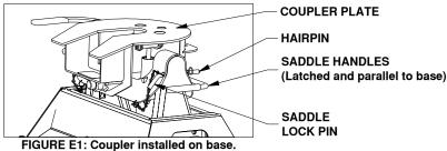
Adjust the resting angle of your coupler plate by rotating the spring on the driver side pivot arm. Pulling the top of the spring away from the cab will increase the angle of the coupler plate. Set the angle of the coupler so that head will tilt away from the cab when coupling, see figure E2. Tighten the 1/4" nut once the springs orientation is set.
