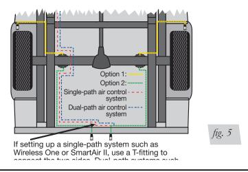
Whatever the chosen location, make sure there is enough clearance around the inflation valves for an air chuck.
