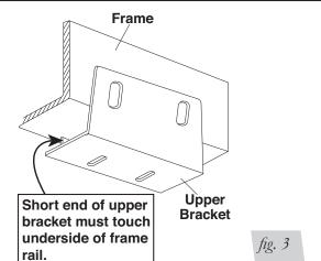
2. Put the upper bracket into position on the frame rail and drill one 1/2" hole in the side of the frame rail (Fig. 3).
