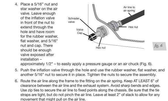
7. Cut off the air line, leaving approximately 12" of extra air line. A clean square cut will prevent leaks. Insert the air line into the air fitting. This is a push-to-connect fitting.
