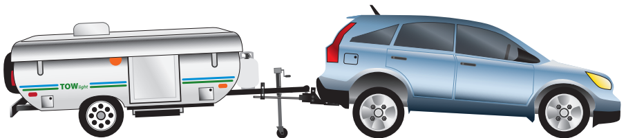
Figure 26 – Raise both trailer and tow vehicle to release tension on spring arms.
