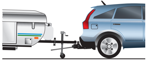
Figure 23 – Lower just enough to lock the coupler
