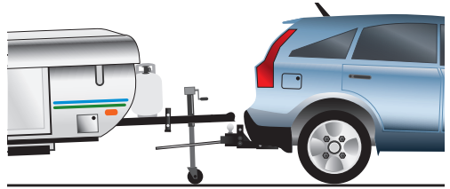
Figure 28 – Uncoupled, ready to move tow vehicle away.
