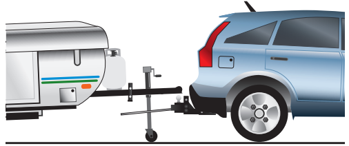
Figure 22 – Position aligned, spring arms in place
