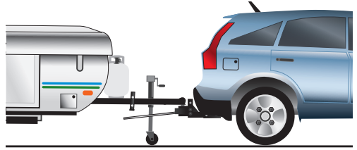
Figure 27 – Lower just enough to open the coupler latch.
