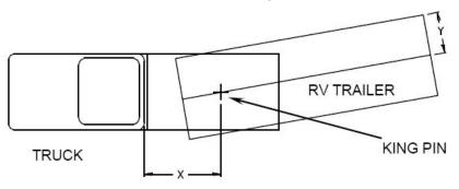
Rule of thumb: The distance from the back of the truck cab to the center of the rear truck axle ("X"), should be approximately 4 inches greater than one-half the trailer width ("Y")
