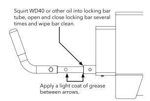
Jaw pins can be removed and greased by removing or unhooking jaw spring and both snap rings. Tap the pin up from bottom. Clean pins and inspect for wear, apply light coat of grease and reinstall pins, snap rings and spring.
