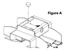
**Note (Read carefully before installing):** Handle can be positioned toward the front or the back if it is found to interfere with the trailer in any way. Verify this before traveling.
