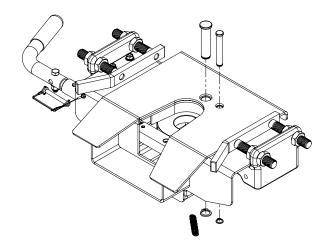
Jaw pins can be removed and greased by removing or unhooking jaw spring and both snap rings. Tap the pin up from bottom. Clean pins and inspect for wear, apply light coat of grease and reinstall pins, snap rings and spring.
