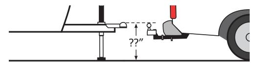
Trailer Coupler Height: \_\_\_\_\_\_ . Set hitch ball to this height. Figure 1
