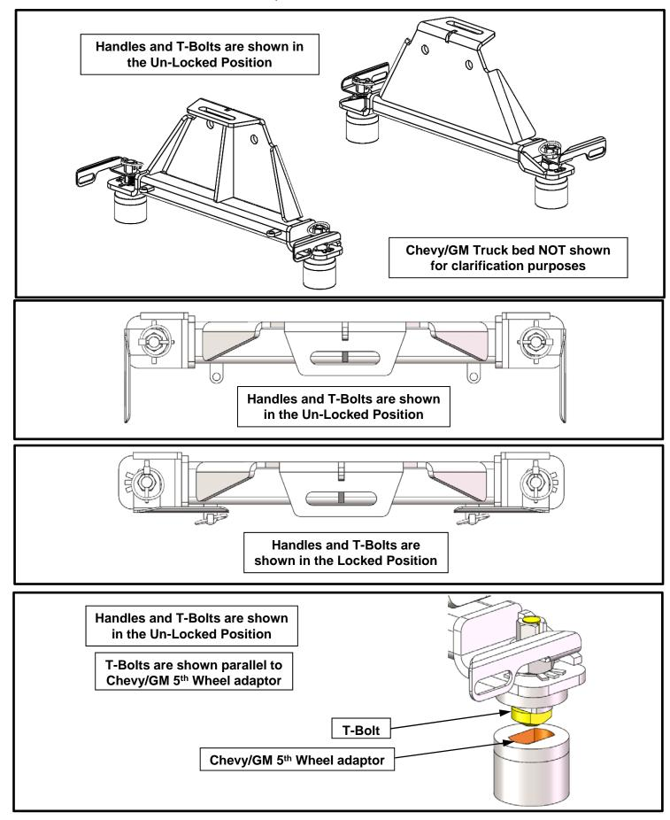
2. Once uprights are installed; turn handles into the locked position. This may require adjusting the T-bolts for a looser or tighter fit.
