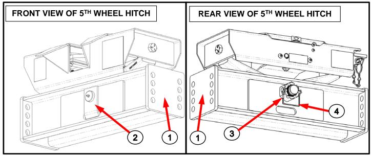
5. Using a grease gun, grease Zerk fitting on plate side of pivot pin
