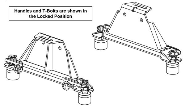
Install the cross member from kit 32998 or 32999 to uprights (#1) using the ¾"-10 bolts (#9) and ¾"-10 nylock nuts (#10). Kit 32998 shown below as an example; kit 32999 installs similarly.
