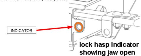
Looking on the back of the Hitch, the indicator should be as shown in the sketch.
