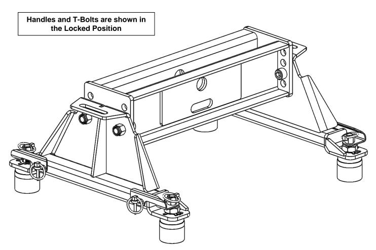
Once the crossmember is installed; make sure the adaptor (#2) sits FLAT with the Chevy/GM 5<sup>th</sup> Wheel Adaptor at ALL 4 contact locations. Torque all four <sup>3</sup>/<sub>4</sub>"-10 bolts (#9) and <sup>3</sup>/<sub>4</sub>"-10 nylock nuts (#10) to 250 ft.lbs.
