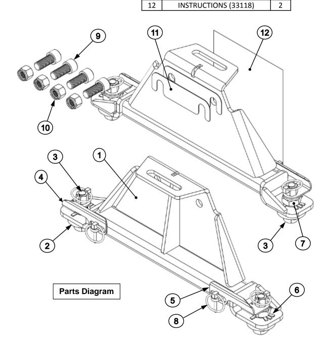
1. Place both uprights into Chevy/GM 5<sup>th</sup> Wheel adaptor installed in your truck from the factory. The handles and T-bolts must be rotated into the Un-locked position.
