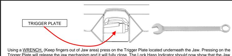
Using a <u>WRENCH</u>, (Reep fingers out of Jaw area) press on the Trigger Plate located underneath the Jaw. Pressing on the Trigger Plate will release the jaw mechanism and it will fully close. The Lock Hasp Indicator should now show that the Jaw is closed.
