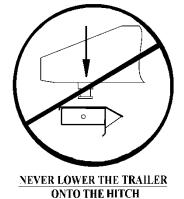
NEVER LOWER THE KING PIN INTO THE HITCH USING THE TRAILER JACKS. THIS IS A VERY DANGEROUS PRACTICE AND WILL RESULT IN THE KING PIN SITTING ON TOP OF HITCH INSTEAD OF INSIDE. THE TRAILER COULD THEN BECOME DETACHED FROM THE TRUCK DURING TOWING CAUSING SERIOUS DAMAGE AND POSSIBLY INJURY OR DEATH.
