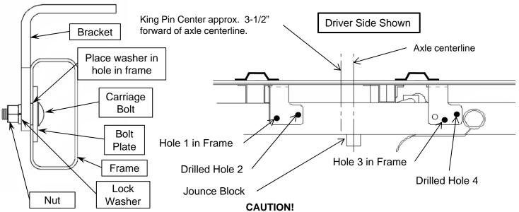
Check for obstructions before drilling. Failure to do so could result in damaged fuel or brake lines, structural members, etc. HUSKY TOWING PRODUCTS, Inc. does its best to communicate tow vehicle manufacturer changes; however, it is ultimately the responsibility of the installer to prevent damage due to installation. All Products limited to Vehicle Tow Rating; see Vehicle Owners Manual
