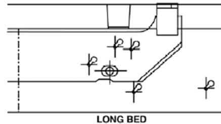
Note: Check cab clearance requirements before installing the hitch. The distance from the cab to the hitch center line is approximately 56" for 8' long beds & 43" for 6.5' long beds.
