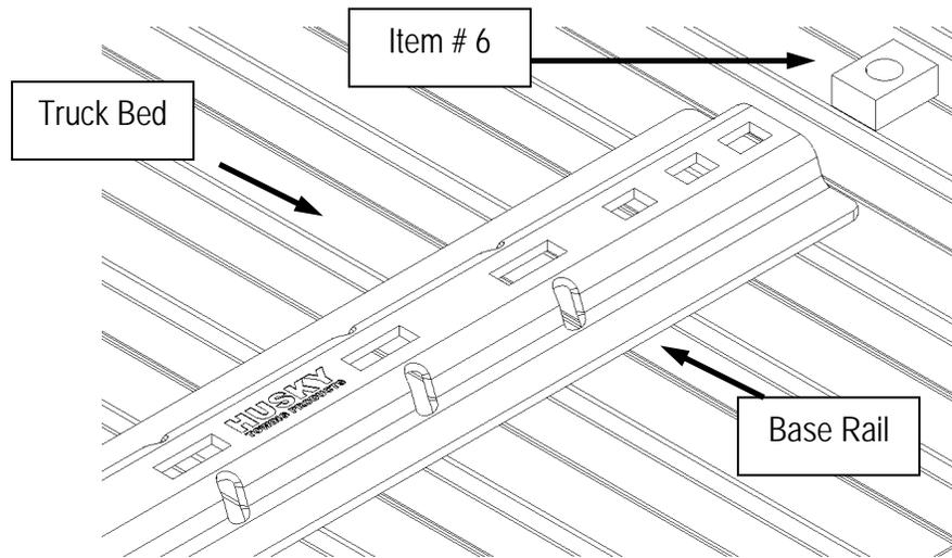
4. If the bed corrugation above the frame is UP, leaving a space above the frame bracket, place a spacer plate (#3) in the bed, under the base rail as shown on Figure 4.
