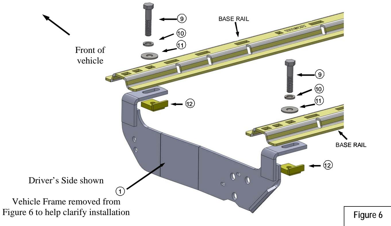
7. Move the frame brackets so that they rest tightly against the flat side of the truck frame and underneath surface of truck bed. Drop the 5/8" hex bolts down through the bed rails and angle bracket. Thread bolts into tapped plates (#12) placed under frame bracket tabs. Securely bolt frame brackets in place. Be sure they are tight against the side of truck frame. See Figure 6. Tighten the 5/8" bolts to 125-160 ft.-lbs. torque.
