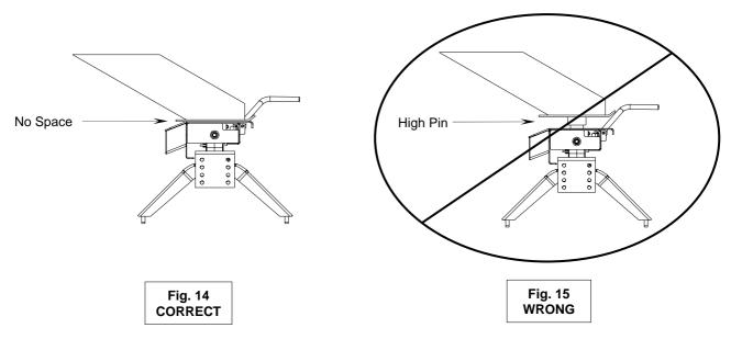
7. Rotate latch for hitch handle to closed position in groove of handle to be sure hitch jaws are locked closed. IF LATCH IS NOT ALIGNED WITH GROOVE IN HANDLE, TRAILER HAS NOT BEEN PROPERLY CONNECTED TO HITCH. DO NOT TOW! Repeat steps 1 - 7 until trailer is properly hitched. (See Fig. 16)
