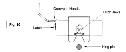
4. With handle in the closed position (See Fig. 10), back truck slowly into trailer. As the trailer king pin enters the hitch it will push the hitch jaws open and extend the handle (See Fig. 11). As king pin completely enters head, jaws will spring closed around king pin and handle will return to the closed position. (See Fig. 12)
