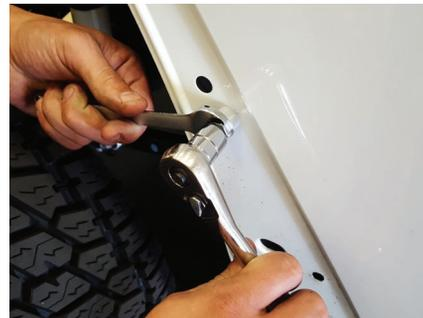
**WARNING:** Over tightening the insert may damage to the thread set tool and / or vehicle rocker panel. Only compress the M8 insert enough to seat it in the hole without rotating.
