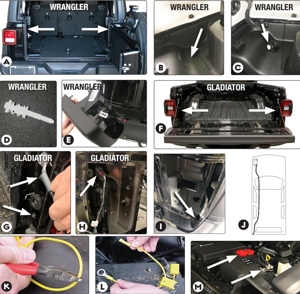
5. Route the harness containing the **green** wire and the 4-Flat down the opening behind the taillight on the driver's side. Route the 4-Flat harness to the center of the vehicle. Route harness containing the green wire underneath the vehicle up through the opening behind the passenger's side taillight.
